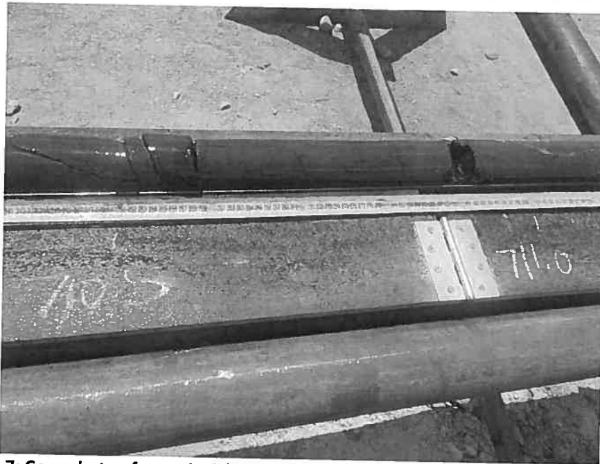
Figure 7: Core photo of organic rich oil-bearing Barney Creek Shale source rock, 710m.
